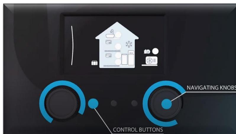
We don't recommend the end user to alter any settings, the most common thing that the end user can change is the settings for DHW scheduling, enabling the heat pump for hot water production within certain intervals in the morning, afternoon or evening. The schedule can alter the set temperatures to which the tank is being heated to i.e. ECO or COMFORT mode or STOP.
